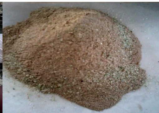
Fig.2 – Glass powder being mixed with sand
